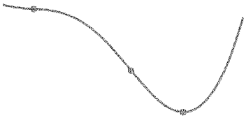
Figure 4.27 The graph for f has no local extremum but has points of inflection where f'' = 0 and x = 2 , and a local minimum where x = 3 . (Example 8)
